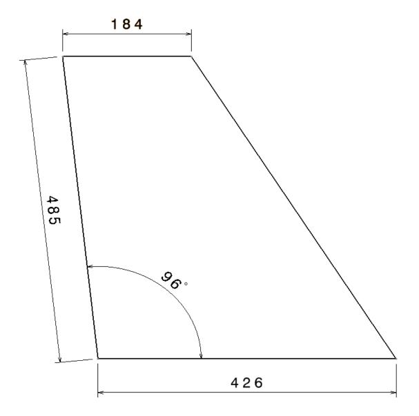
The wing is to be made within a tolerance of +/- 10mm and +/- 1degree from these dimensions.
